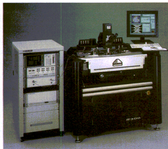
1. Test equipment, such as the S300 RF/microwave probing system from Cascade Microtech, performs accurate measurements on semiconductor wafers that will be used for next-generation communications products.
